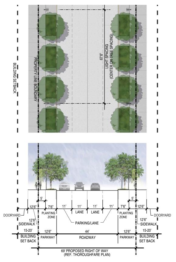
TYPE A : 4 LANE UNDIVIDED WITH PARKING ALLOWED DURING NON-PEAK HOURS TYPE B : 2 LANE WITH 2 LANE PARKING
