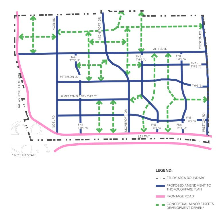
\* THESE MINOR STREETS ARE CONCEPTUAL AND INTENDED ONLY TO ILLUSTRATE DESIRED CONNECTIVITY FOR NEW STREETS. ALTERNATIVE ALIGNMENTS MAY BE APPROVED BY THE DIRECTOR OF PUBLIC WORKS IF THEY PROVIDE EQUIVALENT CONNECTIVITY AND COMPLY WITH THE PROVISIONS OF SECTION 51P-887.115 (STREET STANDARDS) AND SECTION 51A-13.502 (NEW MINOR STREETS).
